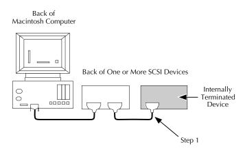
2. Disconnect the end of that cable from the internally terminated device. Do not disconnect the other end of the cable.
